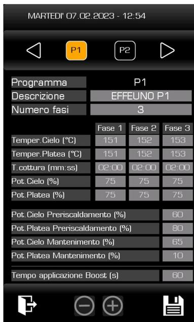
For each of the 30 programs it is possible to modify the name (via an alphanumeric keypad that appears on the screen), the number of phases and, as parameters, the ceiling/chamber temperature set-point, the cooking time, the ceiling percentages /floor and the percentages to be applied in preheating and holding mode.
