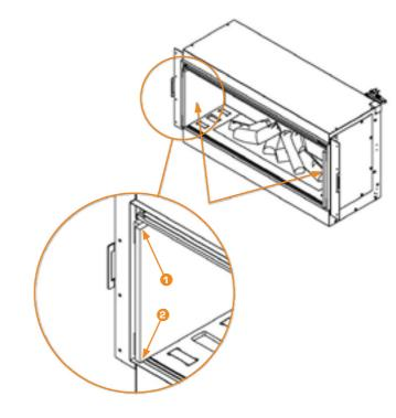
Ensure the front fascia is in the correct orientation, with the "T" on the rear face at the top. Carefully offer the front up to the fixing brackets on the appliance.
