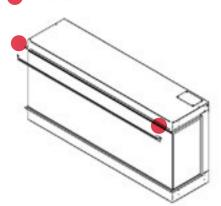
2) Next, gently pull the glass towards you (1), ensuring you have full support of the glass. Lift the glass up and out (2) from the appliance and place the glass on a soft, flat surface on the floor.
